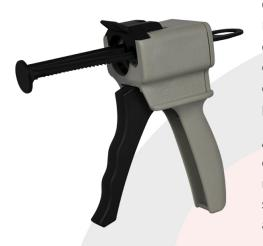
Chemtools<sup>®</sup> DCT-DG8050-110 Ratchet Propelled Twin Piston Cartridge Mixing Gun is specially designed for 50ml 10:1 dual component dispensing cartridges of MMA, Acrylic Cement, Epoxy, or PU. Its heavy duty housing is constructed from high impact light-weight plastic for durability and easy portability, and its twin pistons are designed to provide an even and reliable flow for consistent and precise dispensing.
