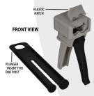
Lift the plastic hatch at the top of the gun and insert the dual cartridge, then close the hatch to secure it in place.
