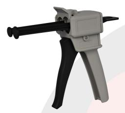
Chemtools® DCT-DG8050-11 Ratchet Propelled Twin Piston Cartridge Mixing Gun is specially designed for 50ml 1:1 and 2:1 dual component dispensing cartridges of MMA, Acrylic Cement, Epoxy, or PU. Its heavy duty housing is constructed from high impact light-weight plastic for durability and easy portability, and its twin pistons are designed to provide an even and reliable flow for consistent and precise dispensing.
