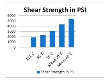
*Result: Lap shear strength reduces with heat and increases in cold temperature. The failure mode was cohesive failure in all above cases.*
